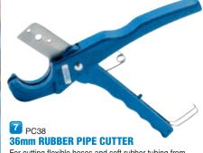
For cutting flexible hoses and soft rubber tubing from 0-36mm diameter. Cast aluminium body with hardened and tempered carbon steel blade and handle clip. Display packed.
