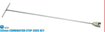
Malleable cast square suitable for 1/2" and 3/4" square heads. 'U' shaped crutch suitable for 1/2" and 3/4" 'T' handled stop cocks. Manufactured from zinc plated mild steel. Display packed.
