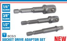
For use in conjunction with any 1/4" hexagon drive unit to drive 1/4", 3/8" and 1/2" square drive sockets. Comprises 1/4" square, 3/8" square and 1/2" square adaptors. Manufactured from chrome vanadium steel hardened, tempered and chrome plated. Each end incorporates a spring-loaded retaining ball for secure socket holding.
