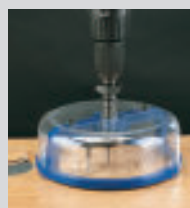
wood dust is self-contained with this hole cutter
