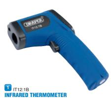
Easy to use 12:1 ratio infra-red thermometer. Compact and portable tool enabling professionals to diagnose heating/cooling problems and monitor the temperature of electrical motors, electrical panels, automotive exhausts and radiators etc; without contact. Manufactured with enhanced optics for delivering supreme accuracy between the temperature range -50 to 550°C (-58 to 1022F), a maximum temperature alarm and a laser
