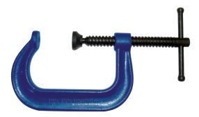
Ideal for heavy duty fabrication and engineering tasks, where very high clamping forces are often required. Sturdy, drop forged steel frame gives a proof load of over 2,000kg (4,400lbs) on the larger sizes. Substantial acme thread for greater applicable torque. The tommy bar will bend before the frame can become overstressed, whilst the swivel shoe applies an even pressure on angled surfaces
