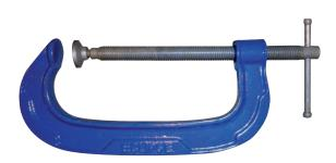
Average clamping force of  $300-800 \mathrm{kg}$  ( $660-1760 \mathrm{lbs}$ ). Guaranteed unbreakable malleable iron frame with a fast action twin start rolled acme thread. The steel swivel shoe applies an even pressure, even on angled surfaces, whilst the tommy bar will bend before the frame can become over-stressed.
