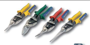
Cuts up to 1.2mm cold rolled steel and 0.7mm stainless steel. Drop forged alloy steel blades give a longer cutting life, whilst the spring loaded handles ensure a fast, smooth cutting action
